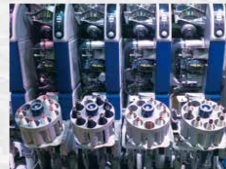
We demonstrated yarn splicing using 4 types of splicers [S.A.S. (Stretch Air Splicer), Hot Splicer, Tencel Splicer and general purpose Air Splicer].
