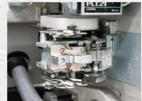
A newly developed "Stretch Air Splicer" solves the technical issues on yarn splicing of spandex yarns which is growing in demand for stretch materials for clothing.
