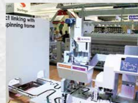
Bobbin Exchanger removes and collects defective bobbins such as half-full bobbins discharged due to yarn quality factors to maximize machine efficiency.
